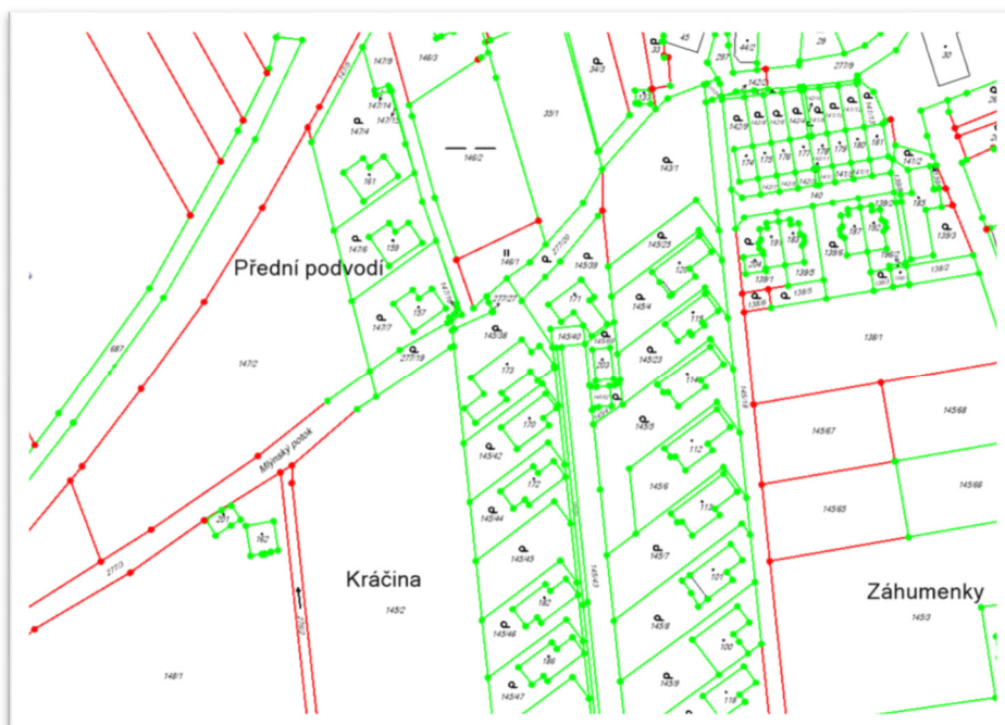
Figure 15: Digital Cadastral Map from Czech Republic with indication of refined and agreed boundaries (green) and less accurate non-agreed boundaries (green).
